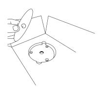
Remove the metal finishing disc and the metal plate with holes and set them aside.
