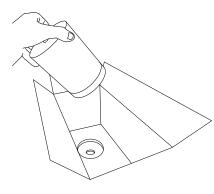
Holding gently the module pull it out of the box ready for set-up and installation.
