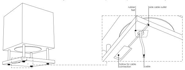
Output cable: Cube 2LV is shipped from the factory with a high performance plug/socket connector (IP68, IP69K) already attached. The plug (male endend) is connected to the bipolar cable of the sound module and the socket (female ended) will have to be connected to the cable going to the amplifier during final installation.
