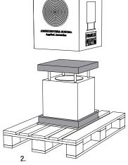
After removing the strapping securing the box to the pallet, lift and remove the box like in the image, leaving on the foam protecting the base.
