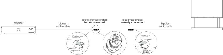
The standard output cable for the Cube 2LV is vertical coming out from below the base. The cable can run horizontally along the hollow space carved below or underground. The Cube 2LV, being a passive subwoofer, requires a proper set-up via an amplifier with DSP on board.
