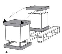
Holding the Cube2LV from the concrete body, NEVER from the base, gently turn the module, tilting it into upper position, WITHOUT removing the protective foam.
